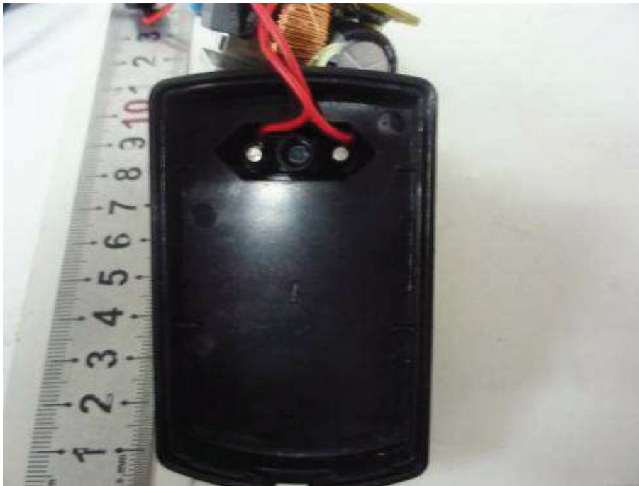
Figure 11. Internal view (Primary wire soldered to pin of plug and hook-in before soldering)
