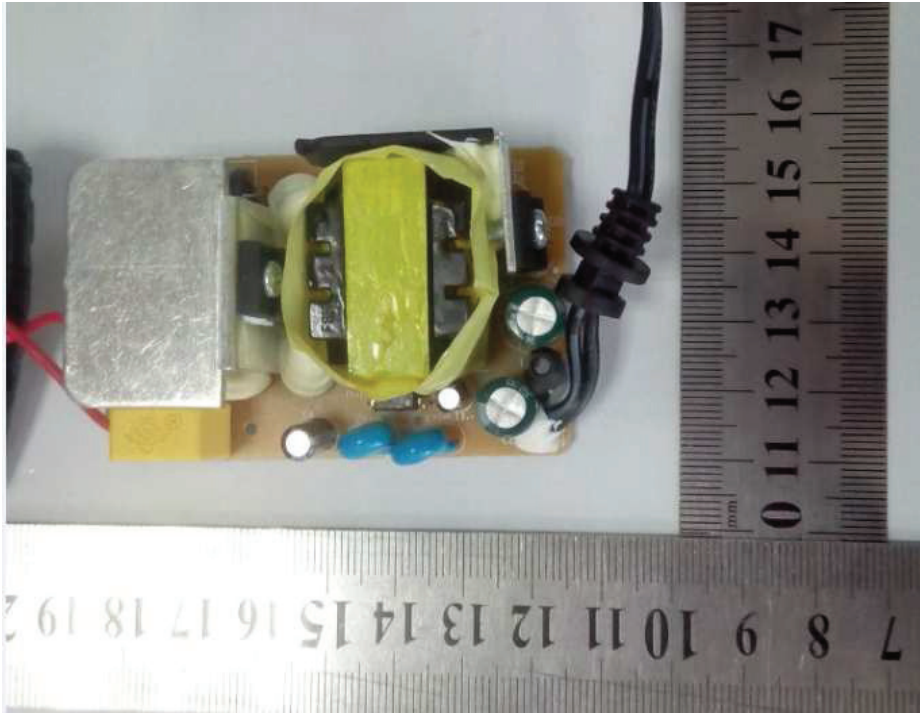
Figure 17. PCB component side of model series B (with two Y-cap in series)
